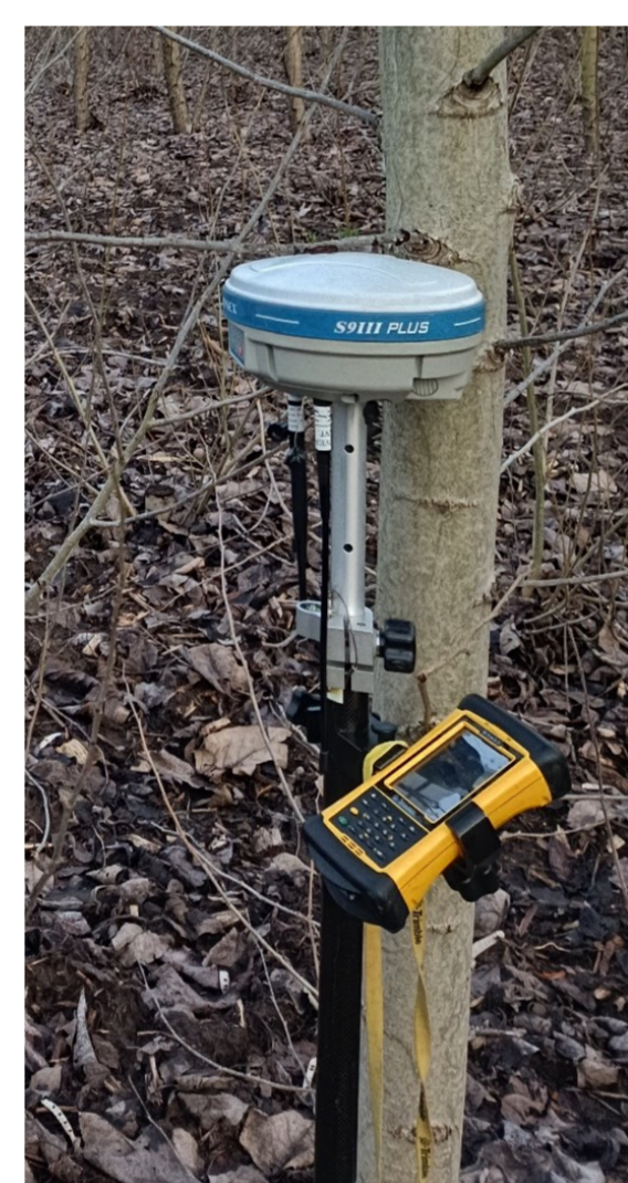
Fig. 2: RTK GNSS Receiver
