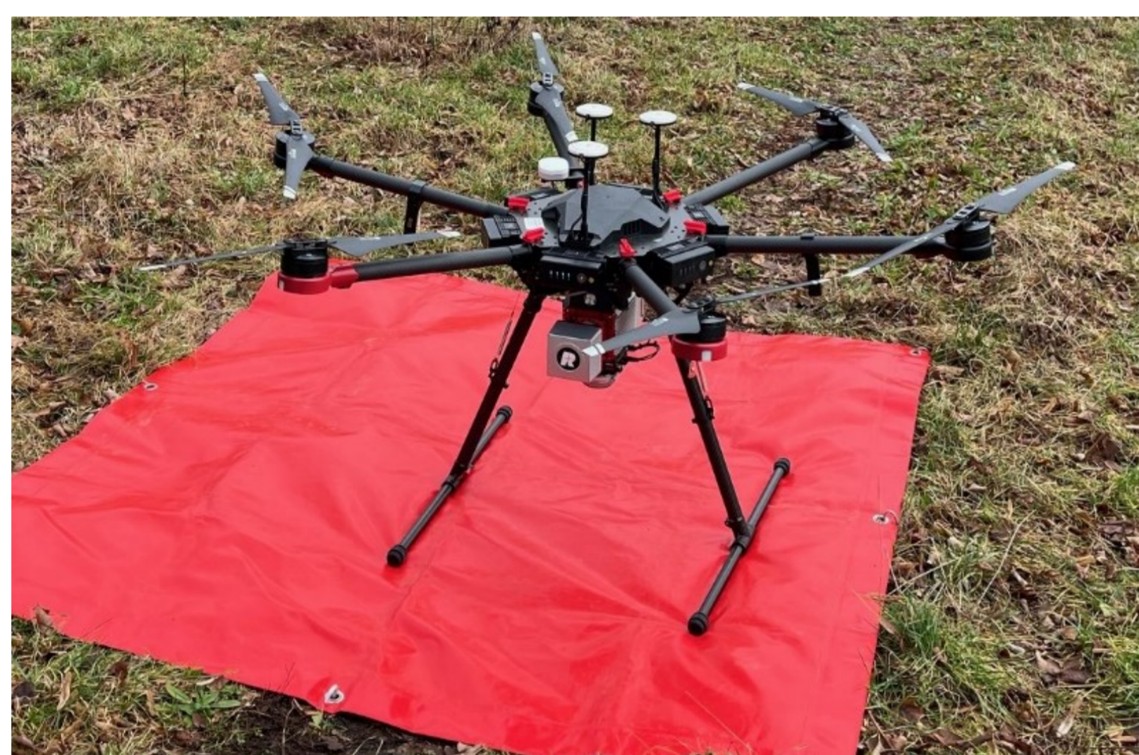
Fig. 1: UAV: DJI (M600), Scanner (RIEGL miniVUX-1UAV)
