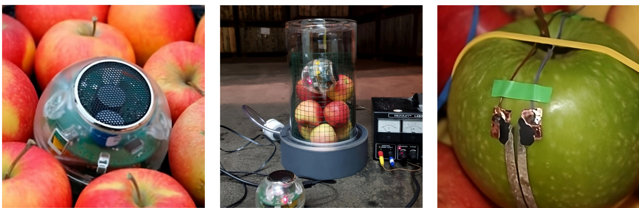
Fig. 1 – Respiration Measuring Sphere RMS88 and Wetness Sensor deployed for real-time monitoring
